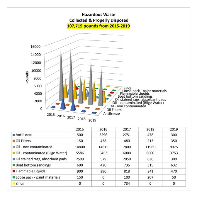
Largest quantities recycled and/or disposed are from non-contaminated Oil and Bilge Water.
